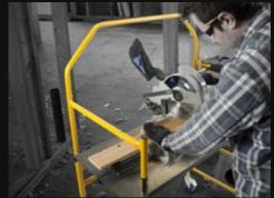
**WORKBENCH**Multi-level working area. Adjust platforms up to the desired level for a comfortable workplace.
